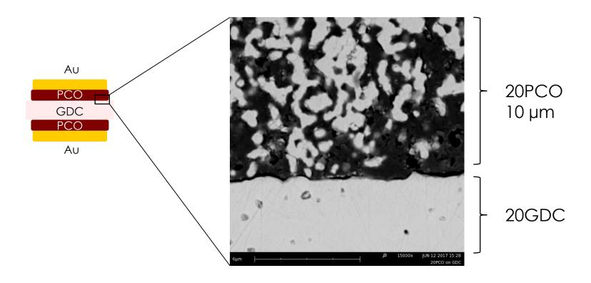
Cathode sintering at 1300°C
